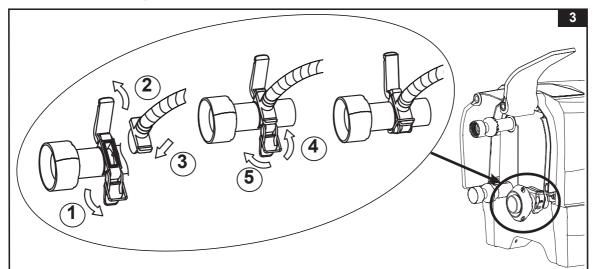
3. Unscrew the air valve cap on the spa tub to reveal the stem in the up position for inflation. Insert the other end of the inflation hose (7) into the valve and turn to the right to lock it in position (see drawing 4).
